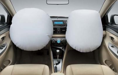
SRS airbags are adopted for the driver's and front passenger's seats. In addition, the body structure efficiently absorbs and distributes energy from frontal and side impacts, while adoption of a high-strength cabin structure helps reduce cabin deformation. The body also mitigates impact energy in the event of a collision with a pedestrian.
